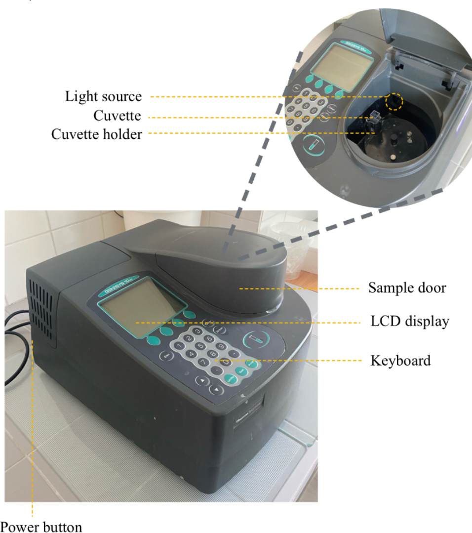
Figure 21: Parts of a spectrophotometer.
