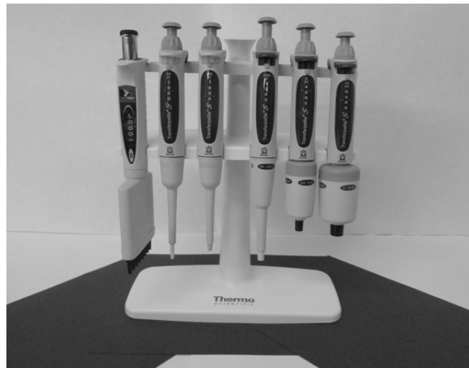
Figure 12: Multi-channel and single-channel mechanical pipettes.
