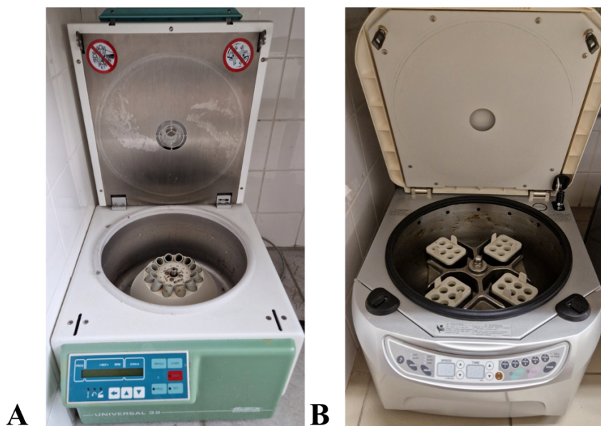
Figure 45: A – fixed-angle centrifuge and B – swinging head centrifuge.
